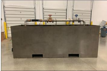
to get the dewatering pump test tank fabricated and on-site. Today, the tank is now onboard NNSY and already in use.
